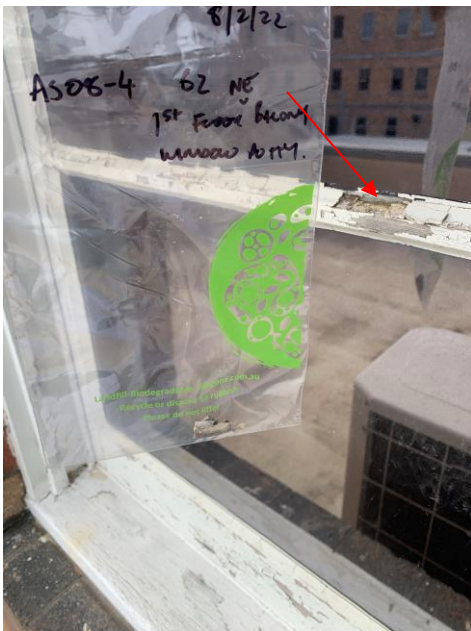
AS08 – 4: No asbestos detected
