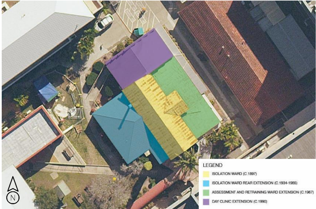
Plate 3.15 Indicative diagram illustrating various, likely phases of development to the Victoria Fever Ward. Source: base map by Metro Maps 2021, diagram by EMM.
