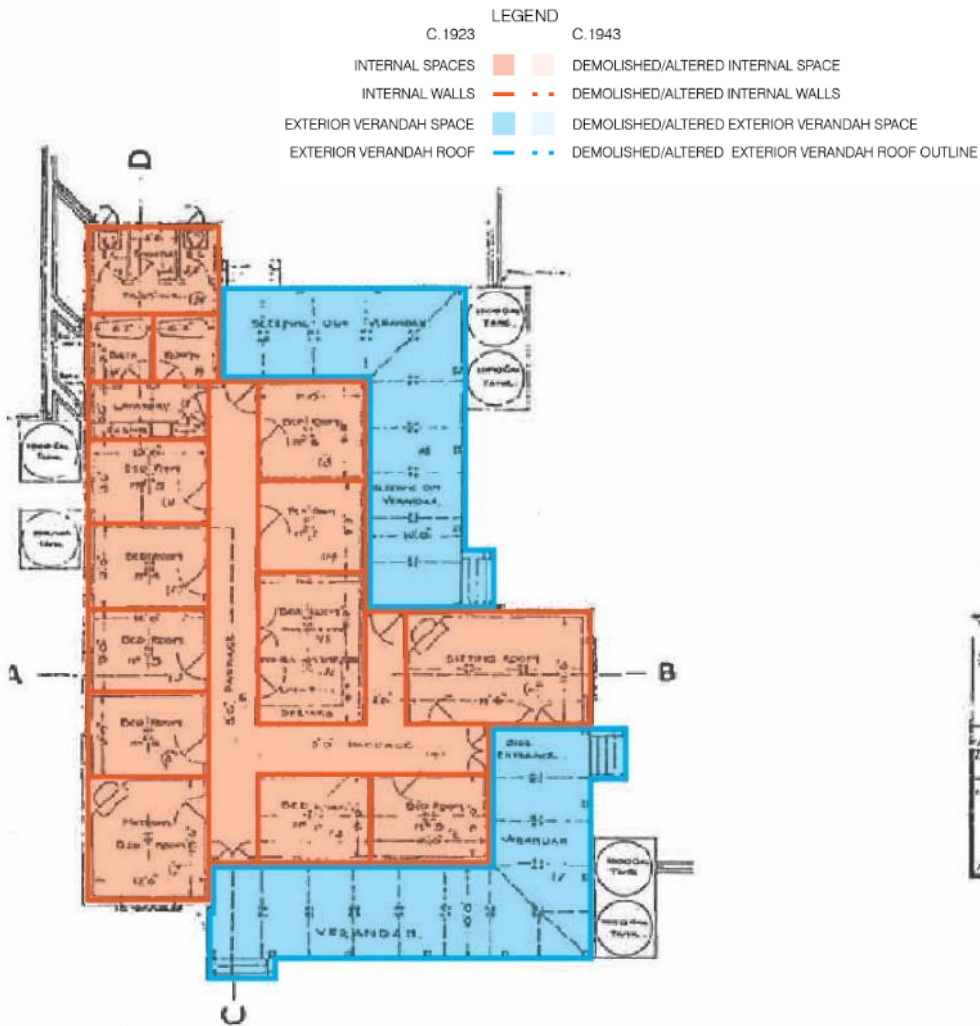
Plate 3.20 Indicative diagram illustrating the proposed alterations, additions and modifications c.1938 (right) to the original c.1923 (left) second nurses' accommodation building. Source: EMM after DPWS 1999.
