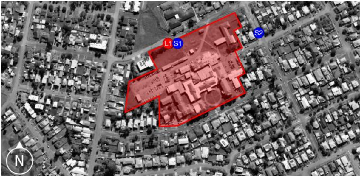
Figure 2: Noise survey locations and boundary of the site.
