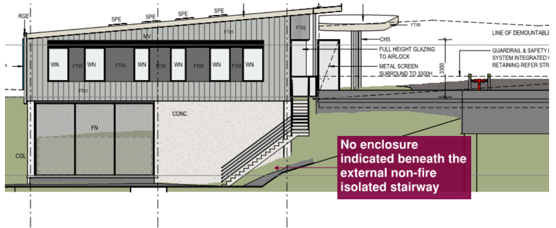
Figure No. 9 – External non-fire isolated stairway on the Eastern Elevation with no proposed enclosure beneath
