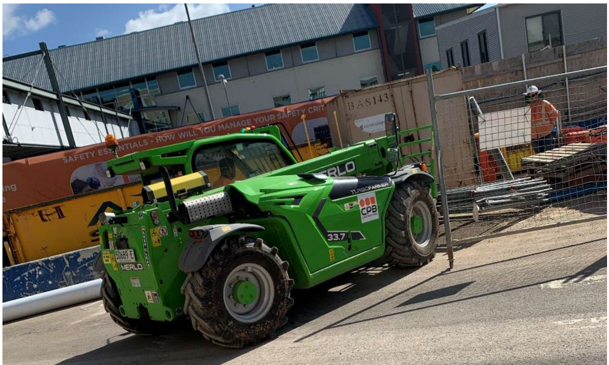
Observation 4 – MERLO Telehandler had a tonal reversing alarm instead of quacker.
