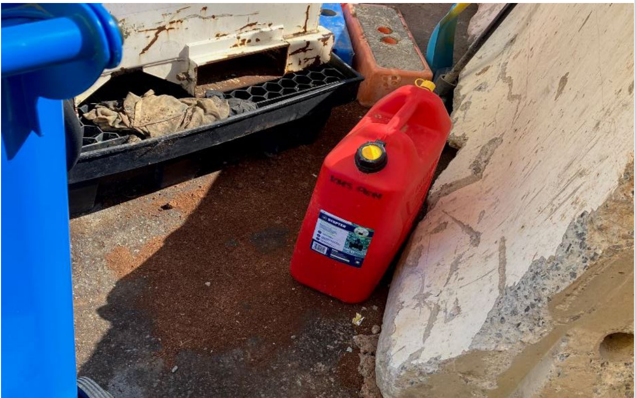
Observation 3 – Unleaded fuel container was not banded or stored adequately.
