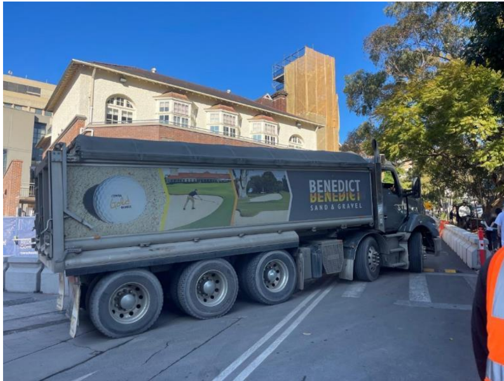
A spoil haulage truck was observed leaving the site with its load covered.
