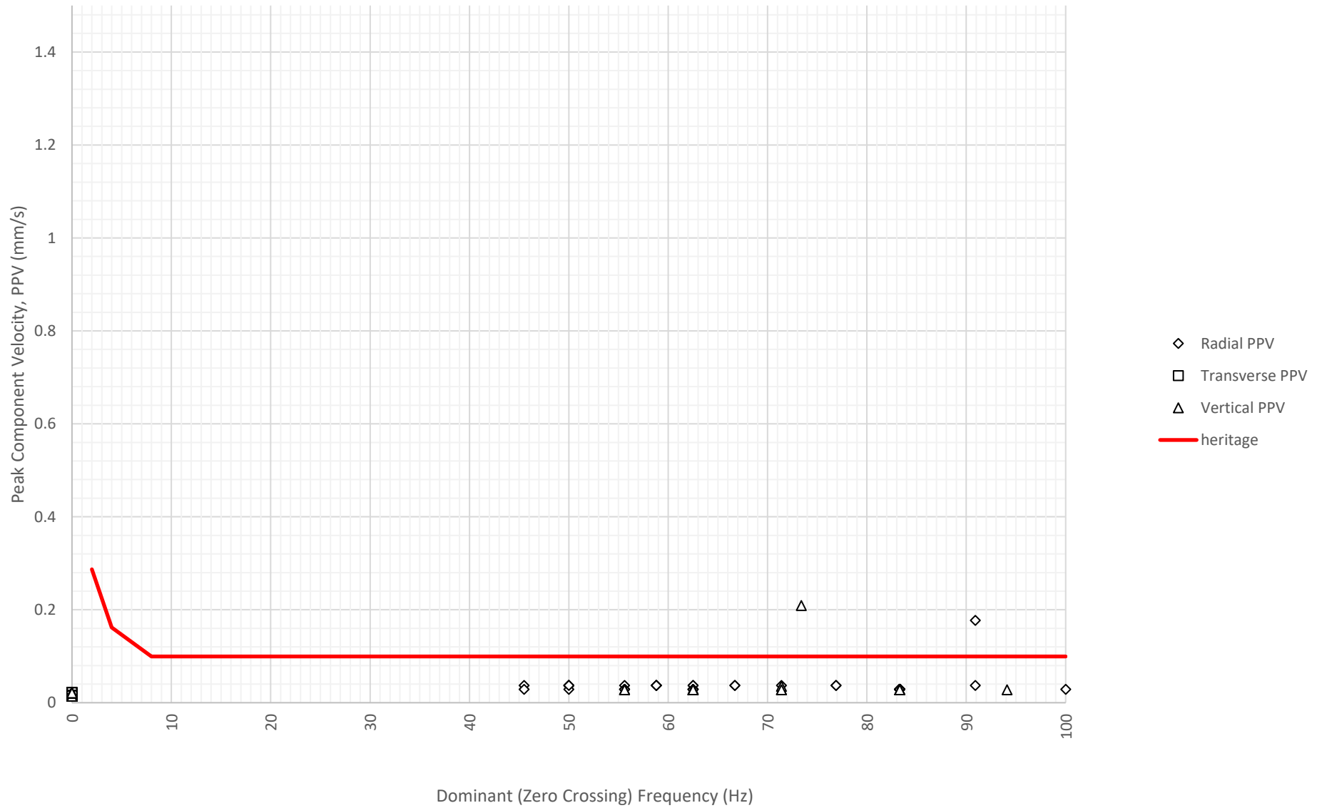
Frequency Content of Vibration Levels at Charles Perkins Centre - Observation Room on 17-08-2024
