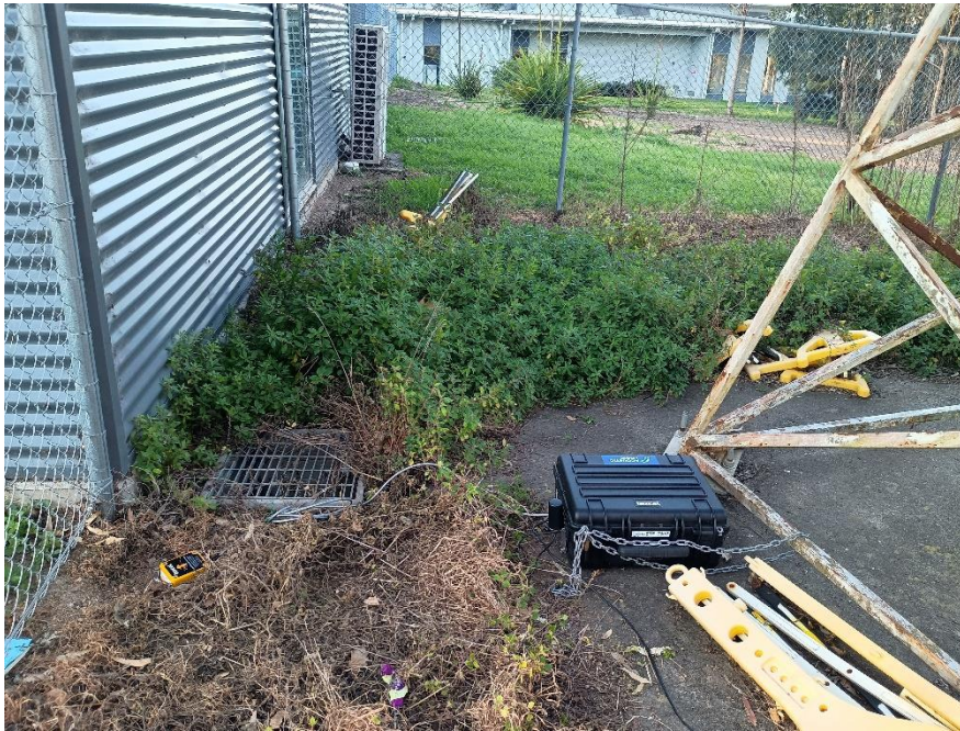
Figure 3. 7900 Vibration Monitor located at North-East of the site (for E1)
